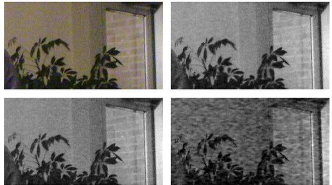
Fig. 1. Portion of an image captured with a Sony DCR-TRV27, and its red, green, and blue channels are shown in raster scan order. The blue channel is the most degraded channel; it has a coarse-grain noise characteristics. The red and green channels have fine-grain noise characteristics.
